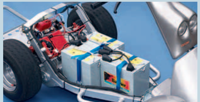
The available space in the conventional design with lead batteries.
