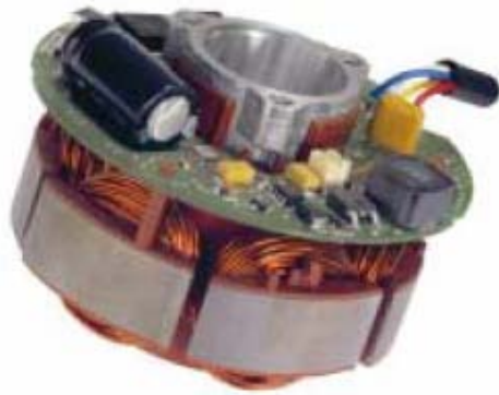
DC motor showing electronic commutation
