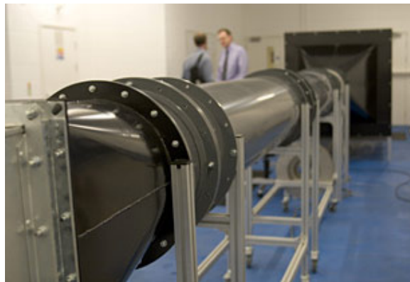
Airflow test rig built to BS848 part 1 / ISO5801:1997.
